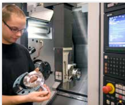
All important components, turned or milled, are controlled for accuracy in our 5-axis CNC co-ordinate measuring machine or other highly accurate specialized inspection or measuring equipment.
