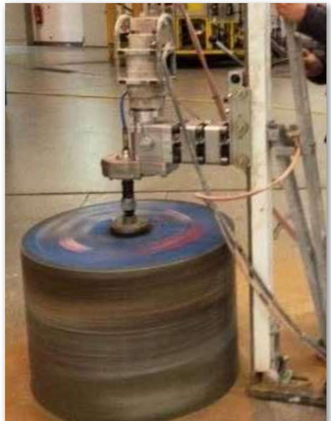
Maximum performance without overloading the diamond tool thanks to superb autofeed
