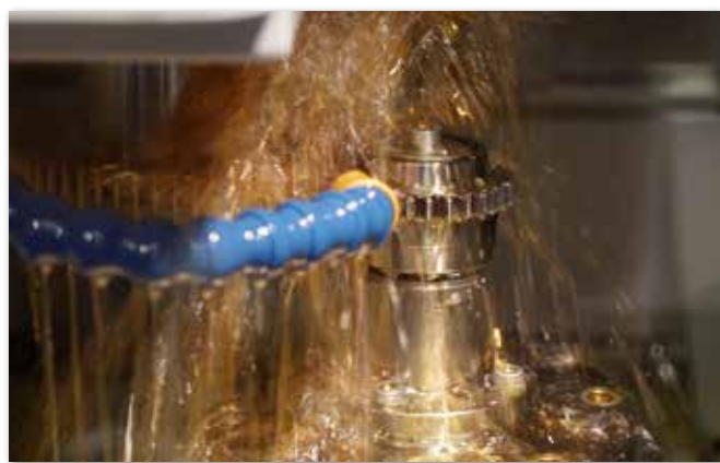
Tractive makes all the gears in-house and grind tooth profiles to very tight tolerances in our ultra high precision gear grinding machine. Aerospace quality is standard.
